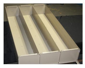
4. Attach 6 Top / Bottoms to sides and backs with flange facing down.
